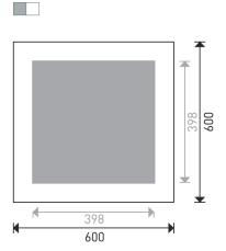
Fire reaction pre and postpainted tiles: A2s1do Release of dangerous sustances: none Flexion resistance: Classe 1
