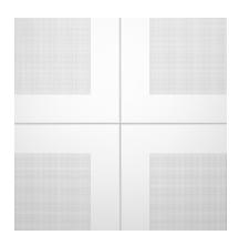
Tile with a non-perforated edge of 100 mm and a perforation pattern in the center  $(\emptyset = 1.5 \text{ mm})$  at an interval of 2.5 mm. Free passage of 6%.
